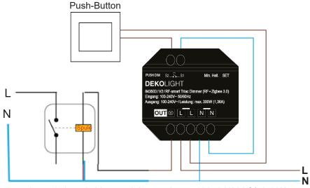
230V Load relay, operation only in switching mode!
