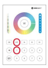
Tip: For remote controls with several zones, you can use the "Master OFF button" to set the minimum brightness for all triac dimmers connected to the remote control at the same time.
