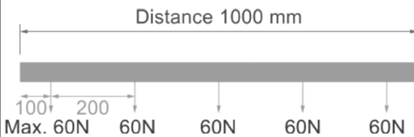
Stromschiene 2000 - 3000 mm / Track 2000 - 3000 mm
