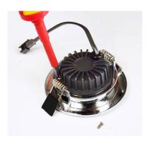
3. Carefully remove the heat sink with the installed LED.
